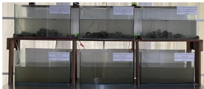
Figure 1. Seawater Samples With (Above) and Without (Below) the Addition of Green Mussels
